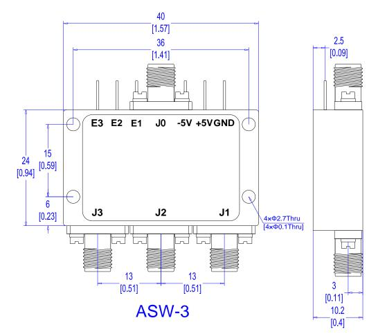
Dimensions are in MM [inches]. Unless otherwise specified. Outline drawing +/-0.1mm: Hole +/-0.1mm
