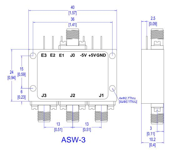
Dimensions are in MM [inches]. Unless otherwise specified, Outline drawing +/-0.1mm; Hole +/-0.1mm.
